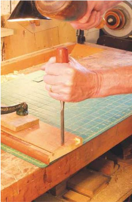
▲ Pic.10 Cleaning the lapped sockets going down first...
